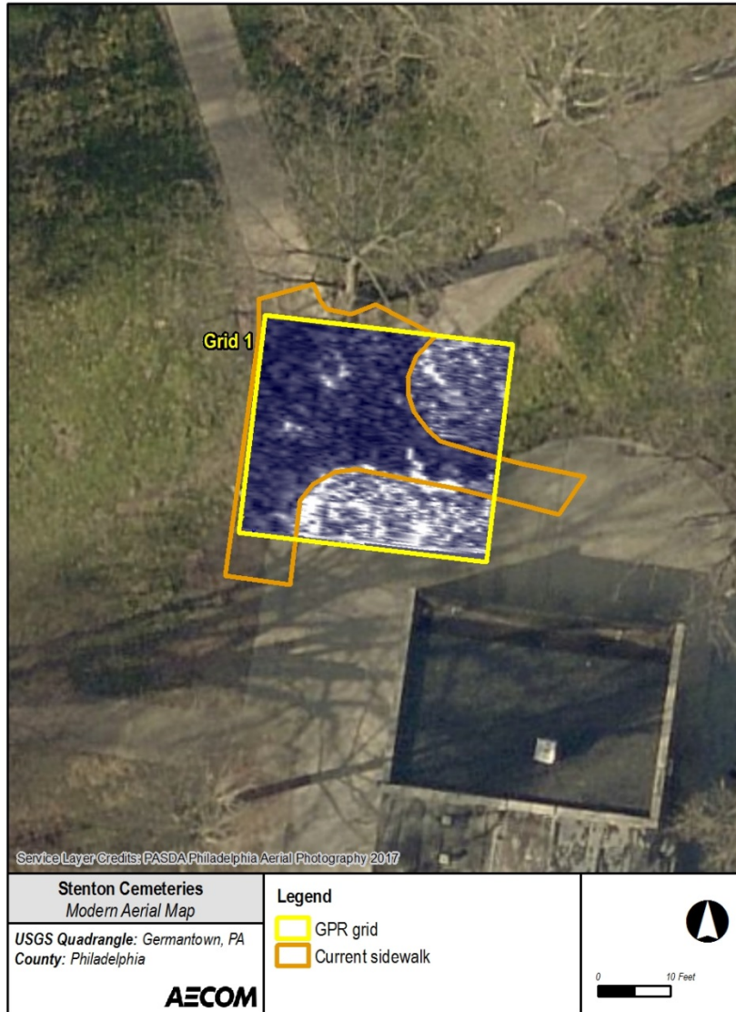
Figure 8 - Grid 1 GPR results. (Note that the aerial predates recreation center reconstruction and related landscape changes. The present-day sidewalk is outlined in orange.)
